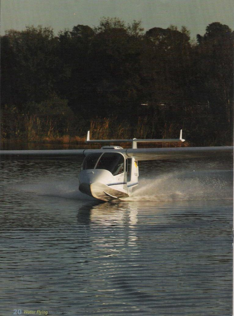
The Gannet (named for a large seabird that soars high to look for fish, then dives for its prey) is a modernday design that incorporates many state-of-the-art composite materials and construction techniques. One of the airplane's unusual features is that after a day of flying, you can disassemble it and trailer it home to your garage.
